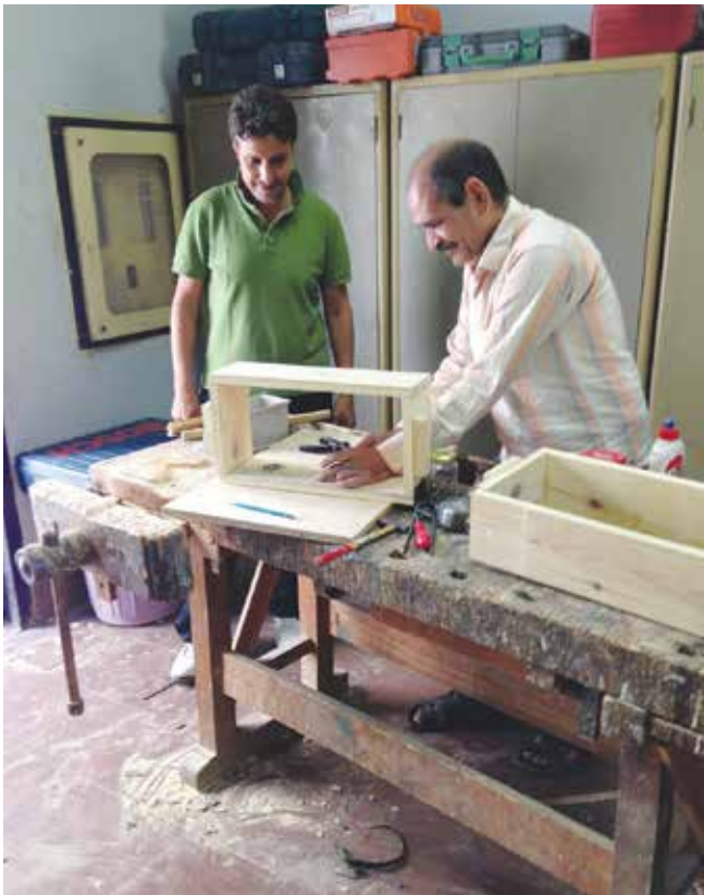
Lotfi and Sami making brick molds. Chicago House. Photo by Ray Johnson
